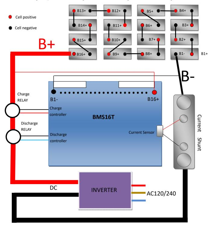
Heavy RED wires are positive of battery pack (B+/B16+), charger and load such as motor, and heavy black wire is negative of battery pack(B-/B1-), charger and load.
